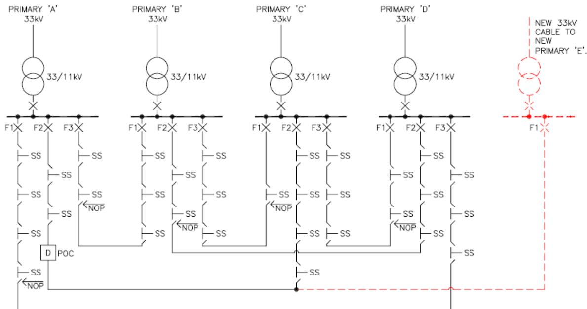
The existing network consists of four 10MVA primary transformer substations and associated 11kV switchgear. A new connection of 4MVA has been requested in the vicinity of F2 from Primary A.
