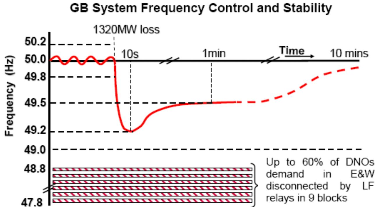
Figure 1 illustrates the frequency control philosophy and frequency stability of the GB power system. In addition, where the initial frequency is close to the lower operational limit of 49.8Hz at the time of a 1320MW loss, the lowest planned frequency would be 49Hz. This would still restrict the maximum frequency deviation to 0.8Hz and provide a 0.2Hz margin above the level where the LFDD scheme is designed to operate and disconnect demand.
