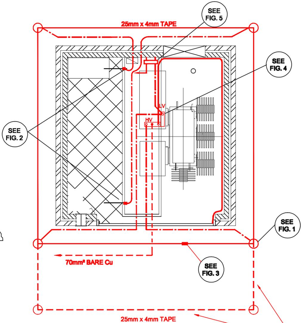
ADDITIONAL ELECTRODE REQUIRED WHEN STEEL DOORS ARE USED. MUST BE INSTALLED OUTSIDE OF DOOR SWING AREA.
