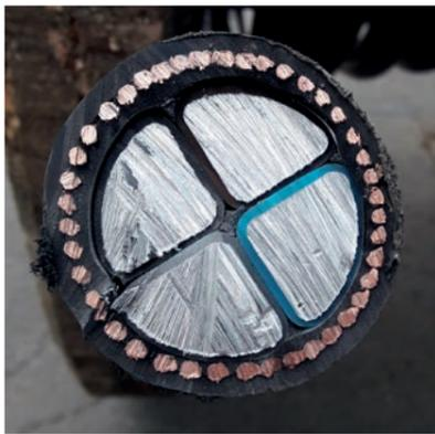
**Figure 4: The inside of a LV 300mm<sup>2</sup> cable used to reduce losses on our network**
