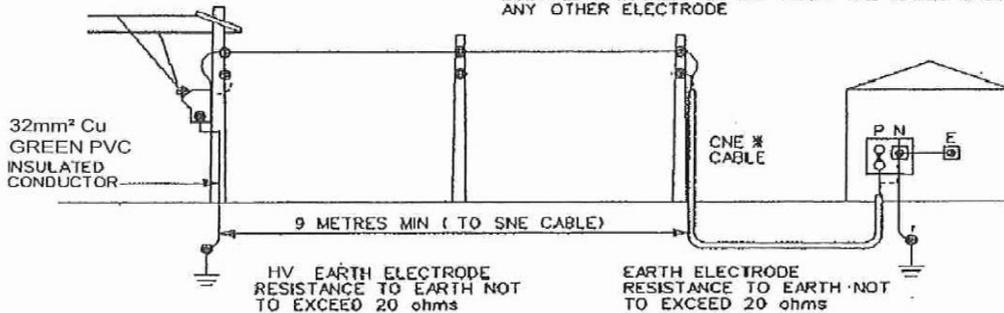
**FIG C OVERHEAD SUPPLY WITH UNDERGROUND CABLE AT SUBSTATION**
