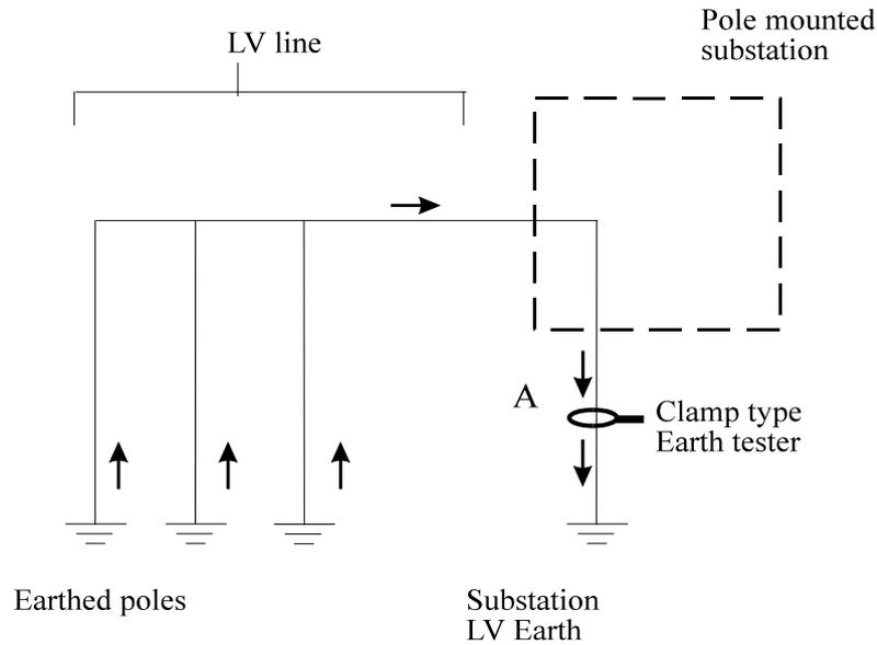
**Figure 1.2.4: Equivalent Circuit of a Loop Resistance Measurement**
