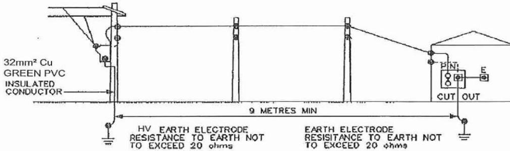
**FIG B OVERHEAD SUPPLY WITH UNDERGROUND SERVICE CABLE**
