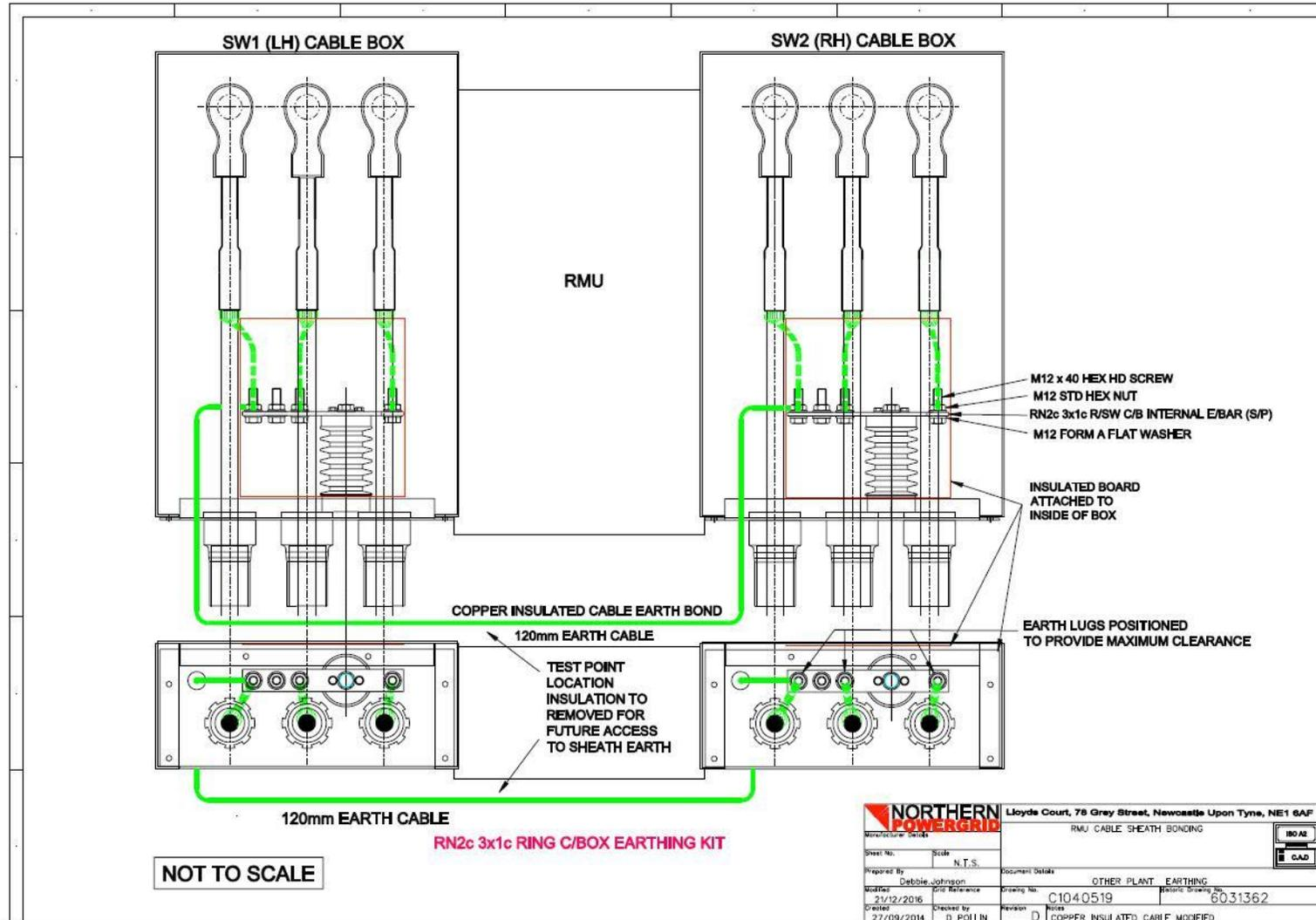
**3.20.9 Cable Sheath Bonding between HV Cables**
