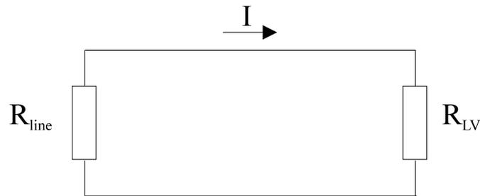
$R_{line}$  is the resistance of the LV overhead earth wire and pole earths, in parallel.
