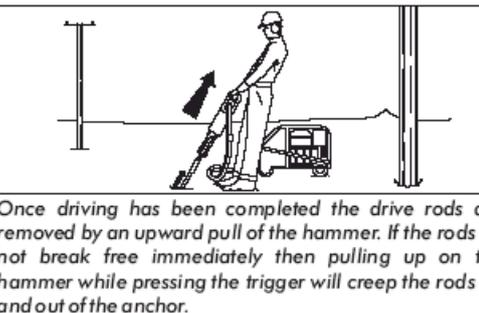
Once driving has been completed the drive rods are removed by an upward pull of the hammer. If the rods do not break free immediately then pulling up on the hammer while pressing the trigger will creep the rods up and out of the anchor.
